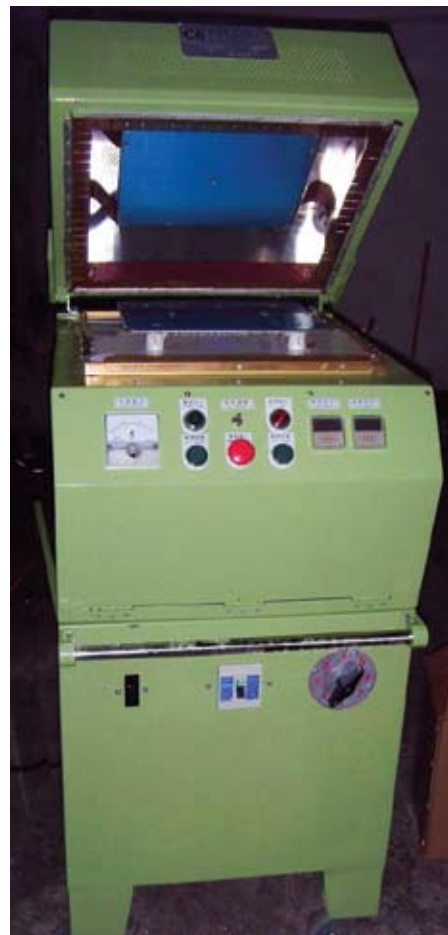
Figure 9: Pre-heater for Melamine Powder
