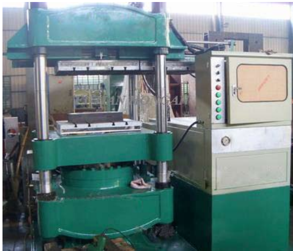
Figure 8: Dense Two Color Melamine Tableware Moulding Machine (good for producing 2-colour tableware)
